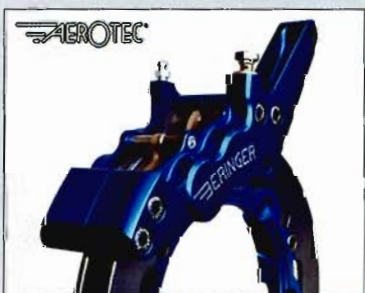
The patented 4D caliper has four 230mm diameter discs instead of the more usual two 320mm discs and two three-pad calipers, which cuts weight and improves power by 20 percent
