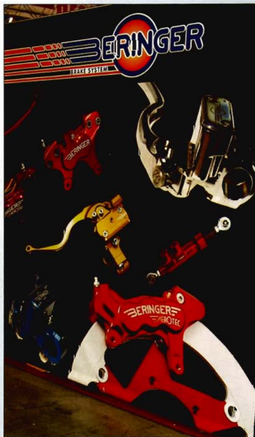
These BR-CC Gold master cylinders are for naked, classic and V-twin bikes and can be used with OEM calipers and discs
