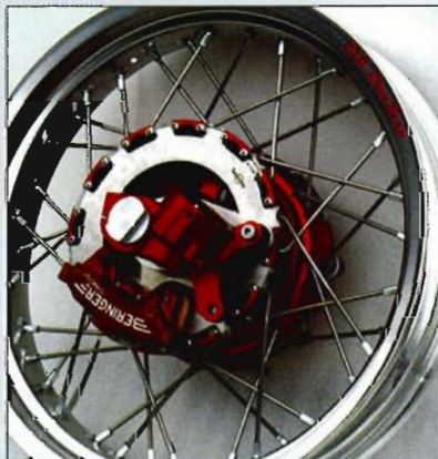
Supermotard twin disc system (above) with two 2-piston Aerotec calipers, two Aeronal floating discs, an Aerotec BRO-10 master cylinder, racing hose and Aerotec pads
