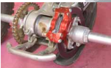
disc + caliper + bracket
