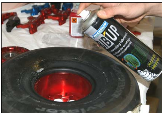
Spray between tyre and wheel with Tire mounting lubricant
