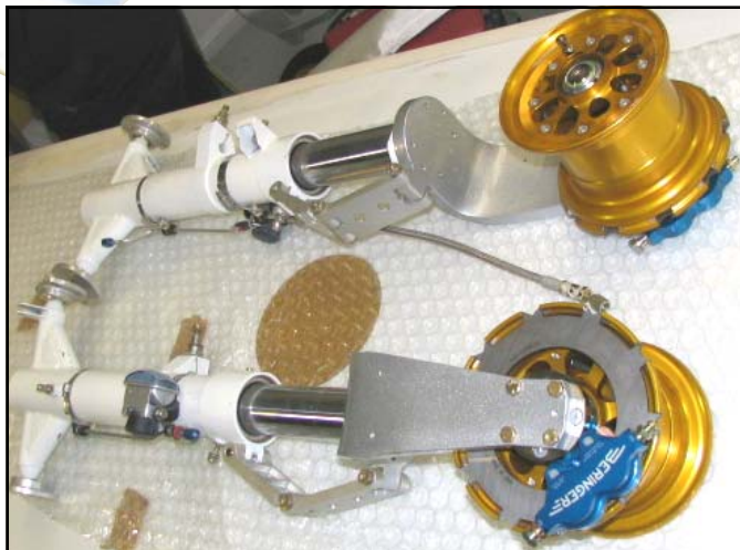
BERINGER Wheels and brakes mounted on Race GLASAIR III landing gear
