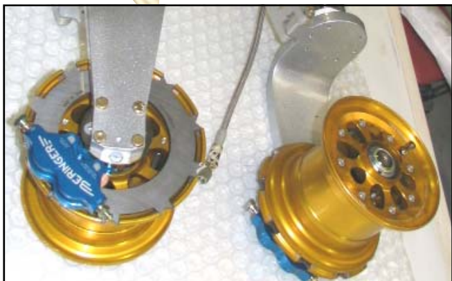
BERINGER Wheels and brakes mounted on Race GLASAIR III landing gear
